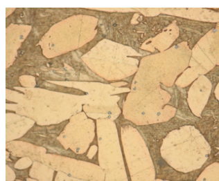
Fig. 1.a) Optical microstructure of B1 sample, x 500; reagent: 25mL HCl + 5g FeCl 3 + 100mL H 2 O
