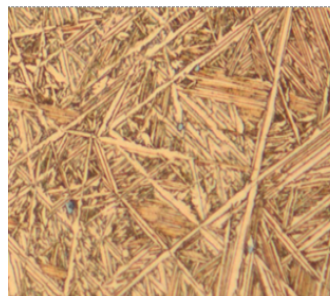
Fig. 4.a) Optical microstructure of B4 sample, x500, reagent: 25mL HCl + 5g FeCl 3 + 100mL H 2 O
