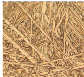
Fig. 5.a) Optical microstructure of B5 sample, x500, reagent: 25mL HCl + 5g FeCl 3 + 100mL H 2 O.
